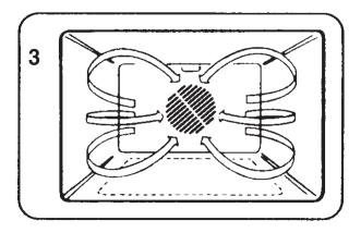
3. **Fan Cooking (Lower Oven)** - the fan oven operates by constantly blowing heated air from an element wrapped around the fan into the oven. This gives improved efficiency and, in general, enables the use of lower temperatures for cooking. It also means that there is less need to be particular about shelf positions and that you can bake at more than one level simultaneously (Batch Baking).
